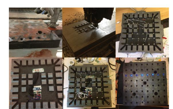
*Digital Paver* is a prototype of a modular concrete paver retrofitted with a motion sensor, LED's and speakers activating the horizontal plane as a medium to interact with users in the physical and digital domain.
