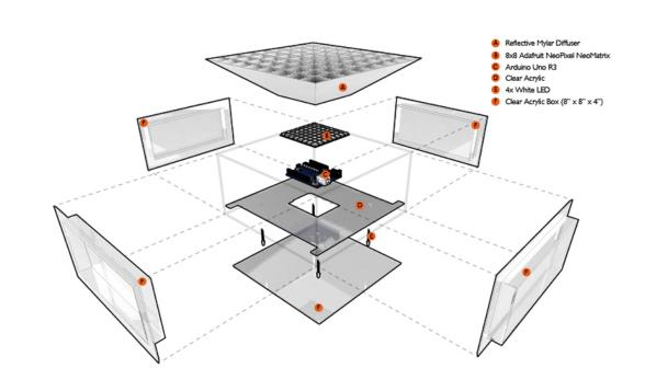
Superblock proposes to embed LEDs and wireless communication into modular acrylic boxes to form a variable resolution display.
