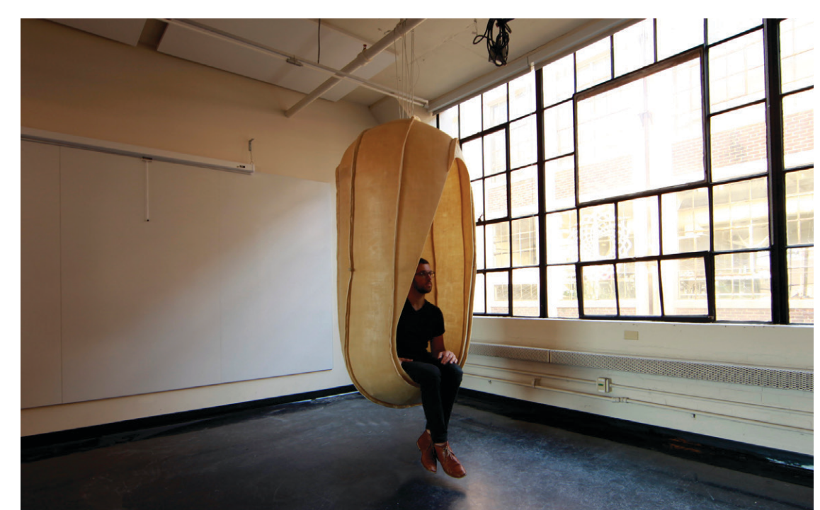
Tough Puff. Research project that recognizes the potential afforded by hybridizing the two disparate fields of inflatables and composites. Using inflatable vinyl bladders as molds for composite production, the expense and inflexibility of the process is radically reduced, with the promise of viably introducing composites to architectural design and building construction.
